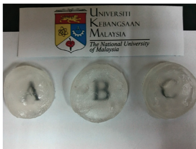
FIGURE 2. Photographs of the cellulose hydrogels (a) CU4, (b) CU6 and (c) CU8
